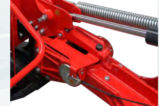
YARIM KİLİT MEKANİZMASI HALF LOCK MECHANISM
