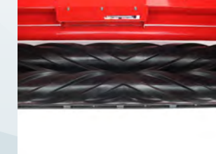
TEK PARÇA POLİÜRETAN MERDANE ONE PIECE POLYURETHANE ROLLER
