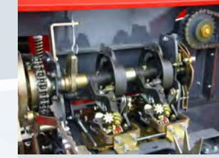
RASSPE BAĞLAMA TİPİ RASSPE THREAD BINDER TYPE
